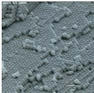
Fig. 2. Electron-microscope photograph of the ordered structure in precious opal, showing its light diffracting 'photon crystals'.
