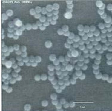
Fig. 1. Electron-microscope photograph of synthesized spherical particles monodisperse silica.
